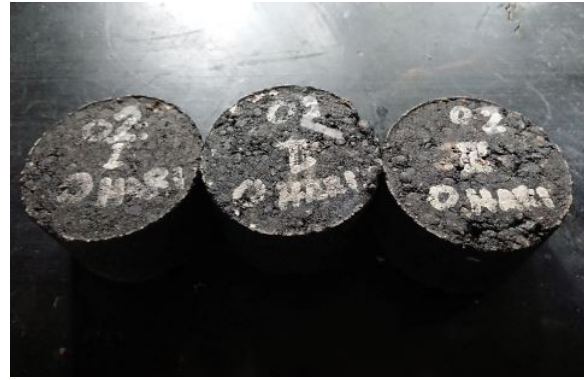
Figure 2: Specimens of compaction of asphalt-concrete mixture
