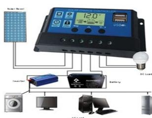
Gambar 5. Diagram System PLTS *Off-Grid*
